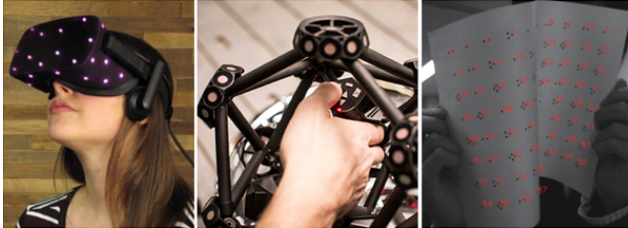
Figure 5: Markers for infrared cameras. (Left) IR LEDs attached to a headset. (Middle) Retroreflective markers, intended to be lit by an infrared light. (Right) Dots of IR ink that absorb light of a particular wavelength and appear as black when lit by an infrared light. Source: iFixit, Creaform 3D and Narita et al. [37].
