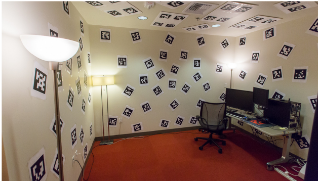
Figure 3: Artificial markers in the form of QR code patterns stuck to the walls. These patterns are easily detected with image processing libraries and have a relatively unique appearance.
