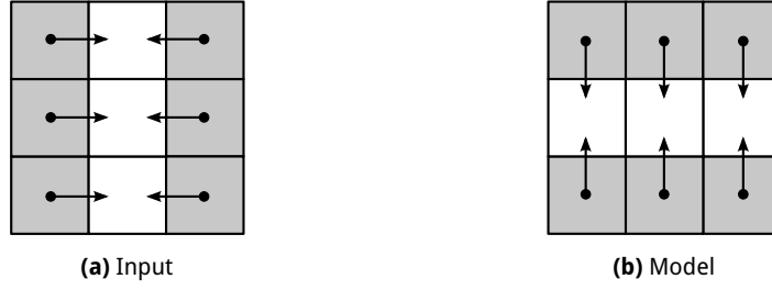
Figure 10: The model and input images are identical 3×3 images, but one is rotated ninety degrees. The gradients are indicated by the black arrows.
