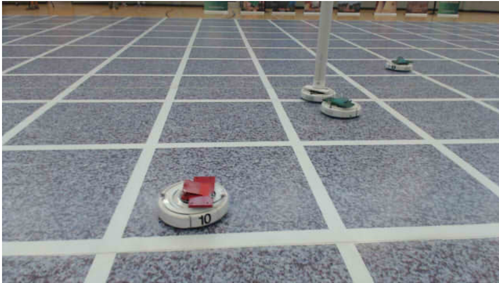
Figure 1: Mission 7 consists of modified iRoomba robots of two kinds, tall obstacles and short targets . In total, there are four obstacles and ten targets. The targets have a front bumper and a top plate (colored red or green) connected to a sensor. When either is activated, the robot will turn a programmed angle and continue in a straight line. Participants must exploit this behaviour to guide the targets across a designated edge of the arena.
